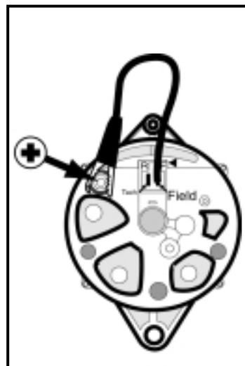
If the alternator fails to generate voltage during field testing, a malfunction of the alternator is likely. Contact your local alternator repair shop or Balmar's technical service staff for recommendations.
